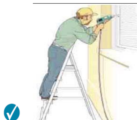
Correct – steps facing work activity
